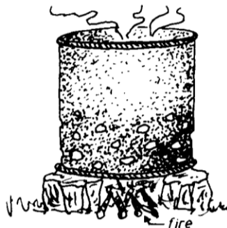
OLD OIL DRUM INCINERATOR holes in side & bottom
