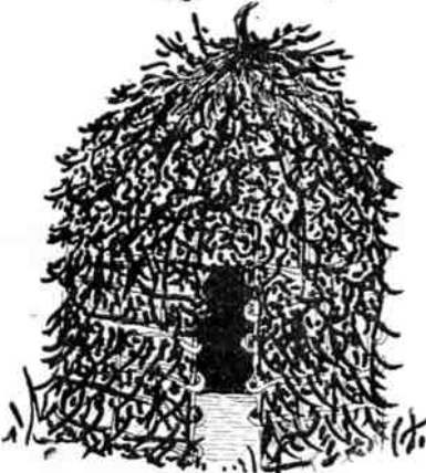
A British Columbia Cedar Lodge, suitable for a short camp. Diameter 7'; side wall, 3'; 24 verticals, 6 horizontals. Description by Assistant Scoutmaster A. W. Morrison, 17th Vancouver. Drawings by B. Morrison.
