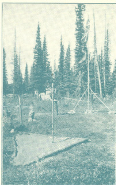
Plan some camp gadgets that instruct. The above group, of the 10th Calgary, include a wind gauge, a sundial with style at angle of lat. 51, and one with style at 96, for checking with one another to show daily variation of sun's circle.
