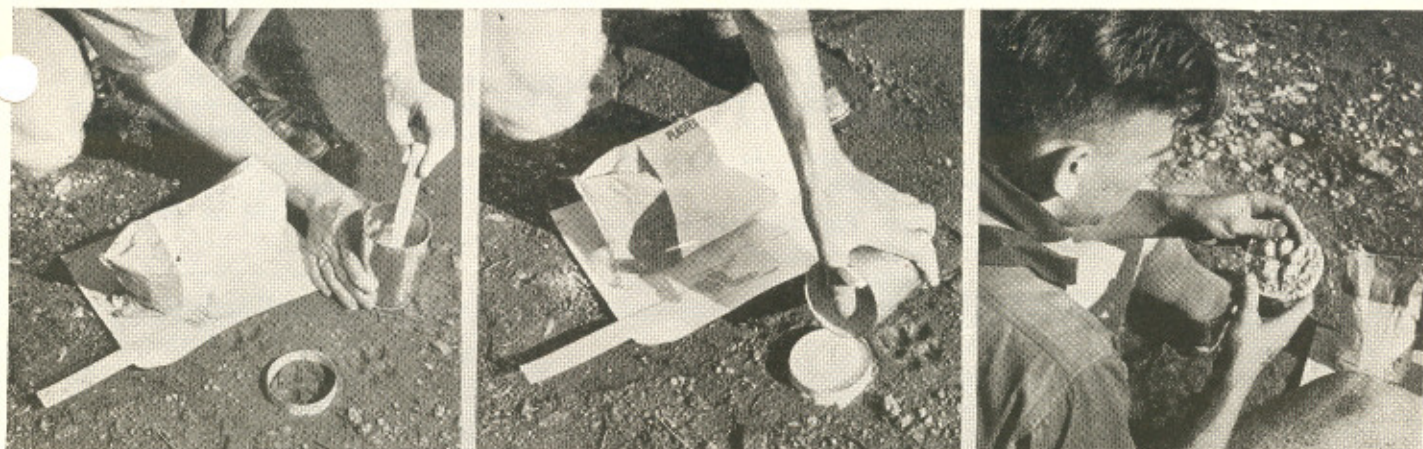
Plaster cast making is a simple operation, which, with a little practice soon brings proficiency. Left shows the cardboard collar around the track; centre, pouring in the mixture; right, examining the finished cast.
