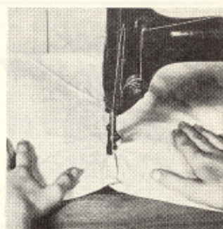
To make flat fell, line up the edges, then sew \frac{1}{2} " in. Swing bottom piece under and sew close to edge. Or use instead the even stronger French Seam, in which, in addition to the above, the top piece is swung over, before the final sewing.
