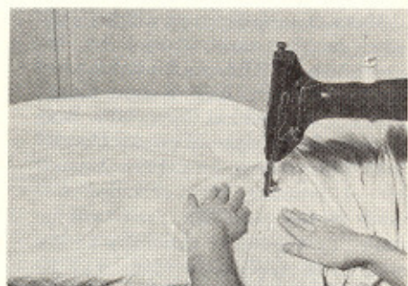
Form sod cloth by folding 11" from bottom as shown in plan. Stitch 1" from folded edge. Hew around tent. Attach heavy \frac{3}{4} " tape pieces to corners, sides, back for tent pegs.
