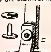
Fastening with copper rivets
