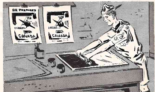
9 Lower the screen and force the color through the screen by passing the squeegee over the surface. Print rapidly so that the screen mesh will not become clogged with paint.
