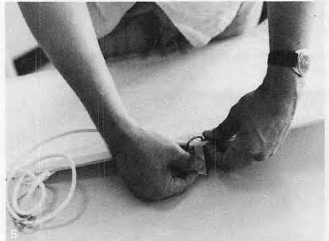
6 On the first two toboggans we ran a rope around the outer edge — to provide strength and to hold the 'D' rings. The rope was sealed to the edge with masking tape. We were not happy with the results and modified our approach on the third toboggan.
