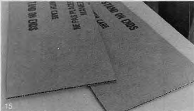
15 On the basis of our experience we decided to use two layers of cardboard for the third toboggan. Because of the curve we cut the bottom layer 4" longer so that we could even it flush after gluing.
