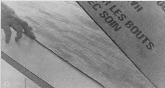
17 The two layers were glued together with rubber cement. For a strong bond, we applied the cement to both faces, allowed them to become almost dry and then put the pieces together after carefully aligning them. Once they are together the cardboard will tear if you try to separate them.
