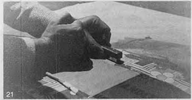
21 We applied a coat of resin to the top and bottom and then stapled the bedsheet to the toboggan. The inset blocks were useful for this. We applied resin, again ensuring that the sheet was firm against the cardboard and that all air was removed.
