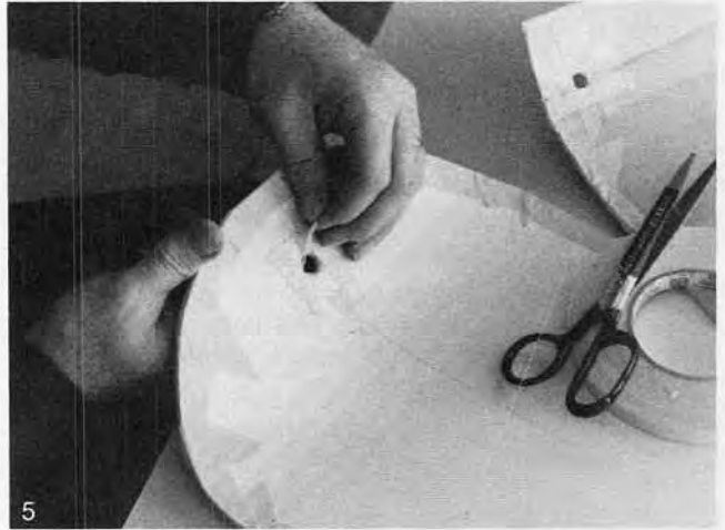
5 We also sealed all edges with masking tape including holes cut in the front curve for ropes.
