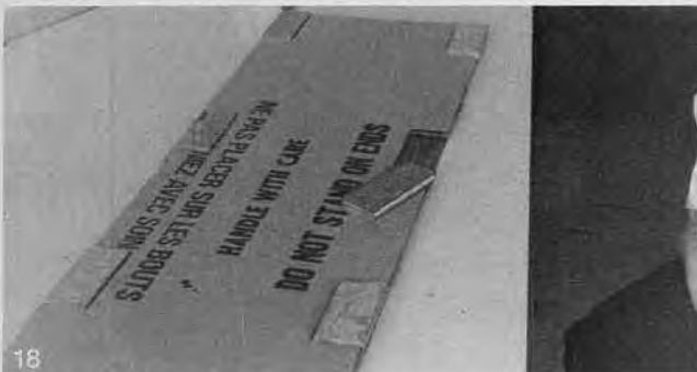
18 Once glued together, we inserted 3/8" plywood blocks along the edge. These were glued in — again using rubber cement.
