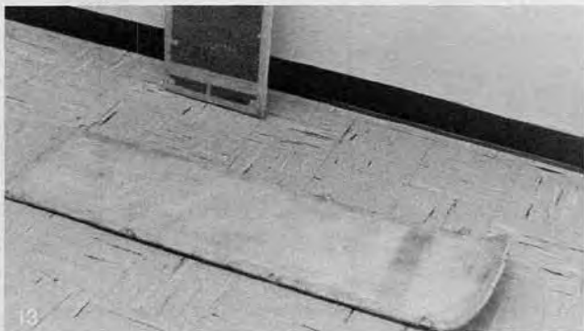
13 This is the toboggan made with foam board, fibre glass and resin. The rounded nose requires modification of the man harness.
