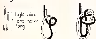
overhand knot as in step 1 of Bowline
