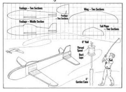
glued together. The fuselage will consist of four thicknesses. Notice on the diagram that the middle two thicknesses incorporate the canopy and tail-fin and that the cone section has been reinforced with an extra thickness at each side.
