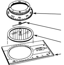
Top of compass housing—with cardinal points on upper rim, degrees on outer rim in two degree portions.
