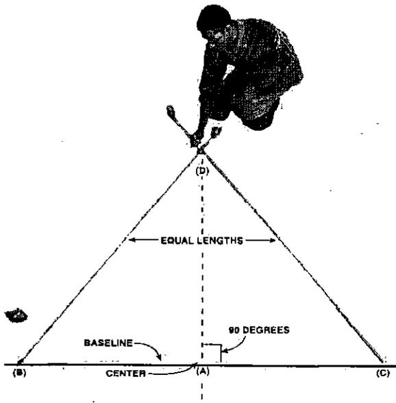
Unless you live in an igloo, you'll probably have to establish right-angle reference lines for one of your home improvement projects. Laying floor tile, building walls and laying patio bricks are a few examples of jobs requiring perpendicular layout lines to get started. The method we're showing is based on simple geometry, but you don't have to do any math to make it work.
