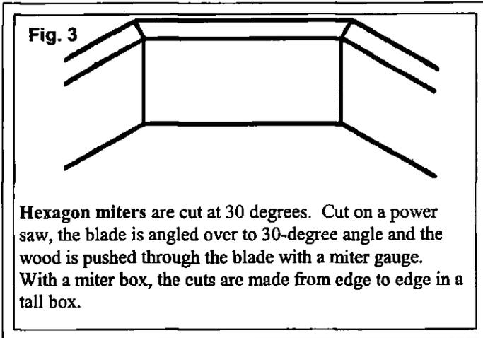
**Using a Miter Box.** Cutting miters using a miter box and backsaw is easy. Before you make the final cuts in good wood, practice a few times. Here are the steps to follow:
