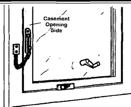
**For casement windows**, use a sliding door lock. This is better than a door chain, because many models can be padlocked. You also can secure a casement window by simply removing the crank that turns the window operator. It is almost impossible to open a window without it.
