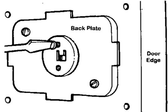
**2. Mark dimensions on door.** Then position and screw on the back plate. Drill the hole for the cylinder partly through the door with another hole for the tang of the cylinder. Insert the cylinder and tang into the hole and then into the backplate, as illustration shows.
