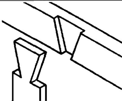
**Dovetail-lap** is a fancy joint where appearance is important. Cut it by hand or with a power saw.
