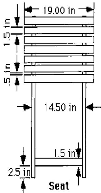
All pieces are cut from a strong hardwood like oak. The Seat Legs and Back Legs are cut from these pieces to form curved pieces. The Seat Leg is 2" wide. The Back Legs are 2.5" wide except for regions that taper to 3" wide to form 1/2" backstops for seat supports. See the seat support detail.
