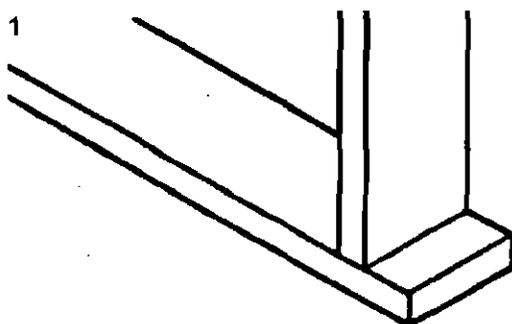
**Butt Joint** is simply the edge or end faces of two boards fastened together; joint is weak.
