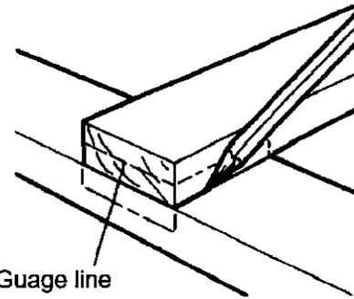
Mark wood to guide saw for lap joint and then make cut. Or use dado blade in power saw.
