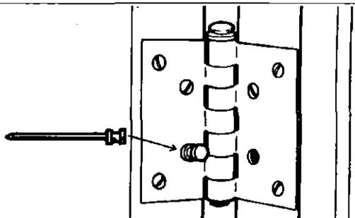
**Exterior hinge pins** are easy for a burglar to tap out and remove the door from the hinges. If you don't want to reset the hinges, you can use the nail gimmick: Remove opposite screws from the hinges. Drive a double-headed or scaffolding nail in one screw hole; drill out the opposite hole so the projecting head of the nail fits this hole. The burglar can remove the pins but the door can't be jimmied off barrels of the hinge or pried off from the exterior side.
