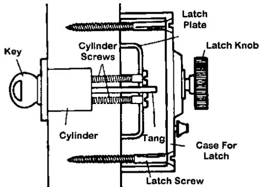
**3. Anatomy of a surface-mounted deadbolt** shows how the cylinder and tang fits through the door and into the backplate and lock. The cylinder is secured in the door by the tang and the backplate, plus two screws driven through the backplate into the back of the cylinder.
