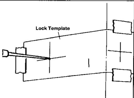
**1. To install a deadbolt,** use the manufacturer's template to locate the hole positions. Tape the template to the door about 10 ins. above the lockset.- use a square to make sure that it is square on the door. Before buying, measure door thickness; locks vary.
