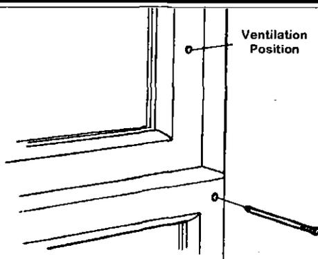
**For double-hung windows**, you can improvise a nail or bolt lock by simply drilling holes through the bottom frame of the window and into the top frame. The nail or bolt is inserted flush into the hole(s). You can space the holes so you can crack the window for air.
