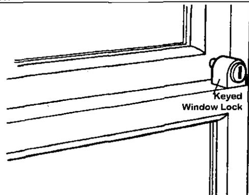
**Win-** **key lock** is best lock type, since the burglar can't open the lock and would have to break the glass and the window mullions in order to get into the house. Some key locks are adjustable so you can crack the window for ventilation without activating the lock.
