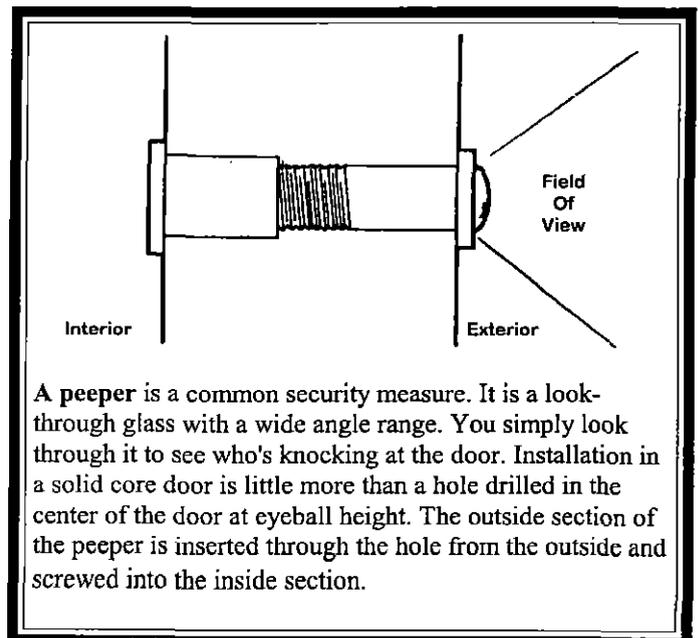
A peeper is a common security measure. It is a look-through glass with a wide angle range. You simply look through it to see who's knocking at the door. Installation in a solid core door is little more than a hole drilled in the center of the door at eyeball height. The outside section of the peeper is inserted through the hole from the outside and screwed into the inside section.
