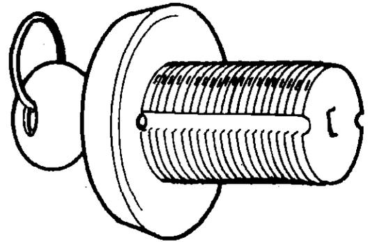
**4. Screw in the cylinder** from the exterior of the door. Special set screws will hold it in position so it can't be removed by a burglar. Then install the strike plate on the doorjamb for the latch bolt. Sometimes, this lock requires only a drilled hole in the jamb to accept the bolt.
