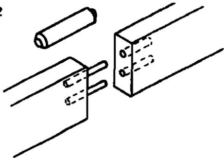
Dowels strengthen butt joints. You must use a stationary drill press or inexpensive doweling jig for this job. You can buy precut dowels with beveled edges and fluted sides which allow trapped glue to escape. End-to-end doweling is called a "splice". About half of the dowel is inserted in each end of the board, but leave room at the bottom of the holes you drilled for excess glue "well".
