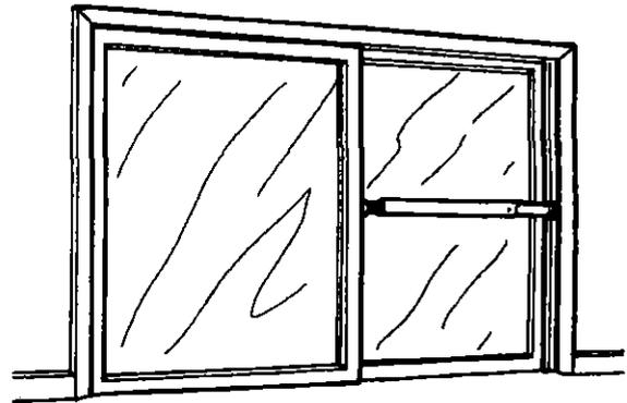
**A burglar bar** on patio windows is deterrent, but a burglar can still force the lock and jimmy the door. Use a burglar bar in combination with the screw trick shown above, plus a window lock. The burglar bar is hinged on one end; there is a width adjustment on the other end.
