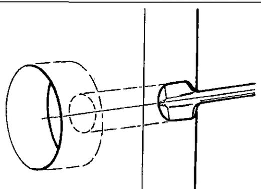
**2. With a hole saw or expansive bit,** drill the hole for the lock first. Then drill the hole for the bolt so both holes form a "unit". The trick is to keep the holes square to the door surface; use a square as you drill for extra accuracy. Deadbolt locks are made for solid core doors.
