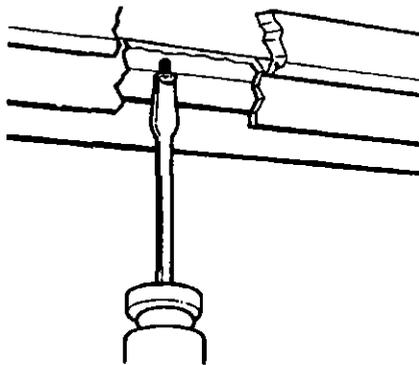
**Patio doors** are easy to jimmy from the outside. Just lift them up and out of the track. The job is more difficult for a burglar to do, if you drive a screw up into the top center of both upper tracks. Let the screw project downward so the door just bypasses the screw.
