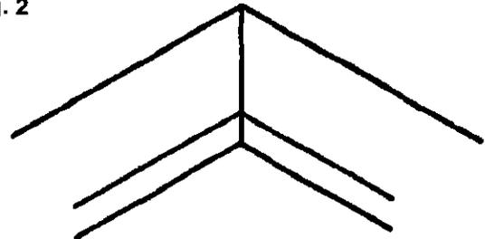
**Miter Joint** can be any angle, but it usually is 45 degrees. The most accurate miter cut is made with a miter saw or in a quality miter box.
