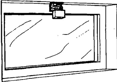
**Basement windows** (hopper type) that open from the top can be secured with a hasp and padlock, as illustrated. Use one-way screws to attach the hasp; this way there is no chance a burglar can break the glass and remove the hasp, if the hasp screws are exposed.
