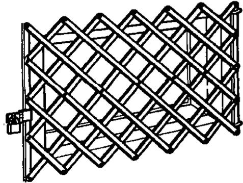
**An accordion gate** offers maximum protection for basement windows, yet is fairly easy to open from the inside in the event of an emergency. The gate is padlocked with a hasp. You also can buy burglar bars or grills that are set into the jambs of the windows.
