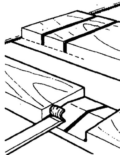
With a sharp chisel, remove the access wood between the saw cuts, as illustrated. Smooth the bottom of the cut with a rasp.
