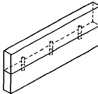
Edges of board must be perfectly square for perfect dowel joints. Apply glue to one end of dowels, then insert dowels into one board. Apply glue to the dowels and adjoining board and tap both pieces together. Clamp.
