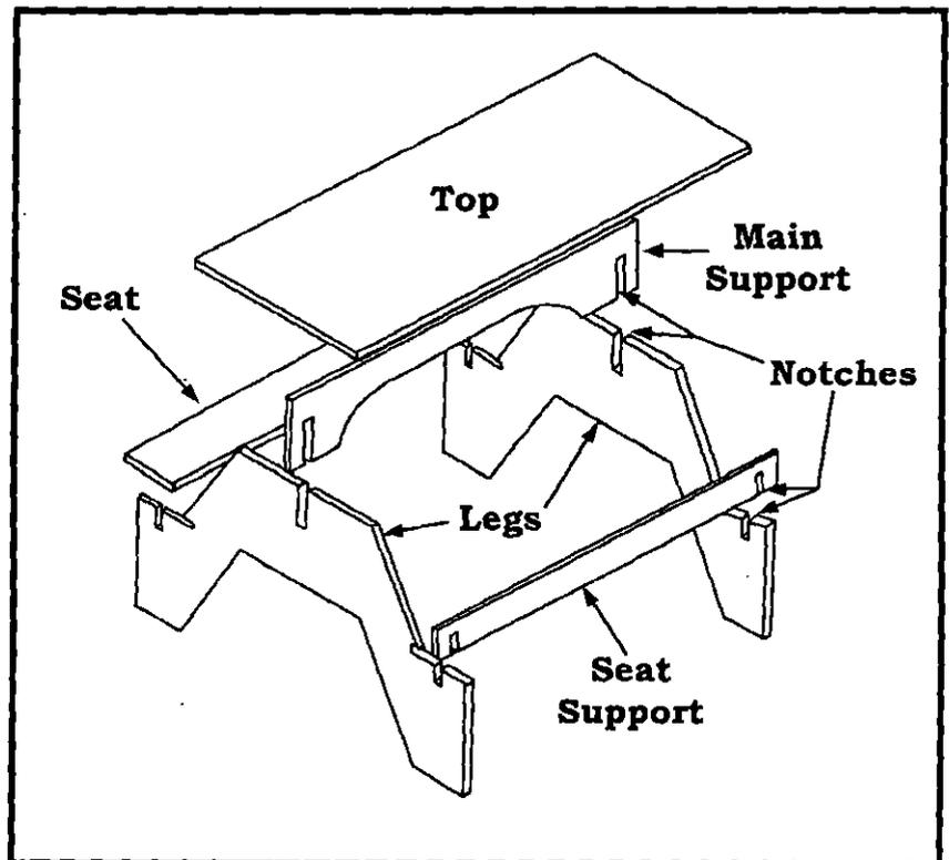
The cleats should be fastened with waterproof glue and rust resistant screws. A good penetrating oil finish (A "MINWAX" type stain/sealer is a good choice) will further prevent splinters and improve the life of the table. Paint will not seal deep enough and will show scratches faster.
