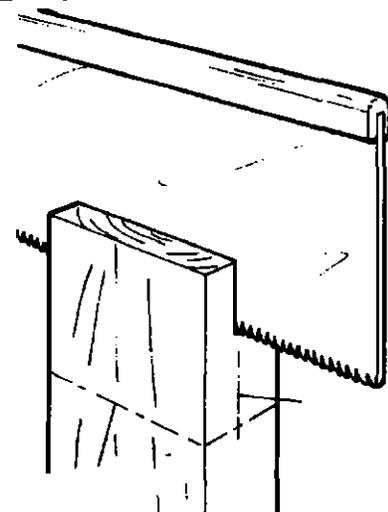
To cut a rabbet joint by hand, use a backsaw guided along penciled cut-off lines. The width of the cut is half the wood's thickness.
