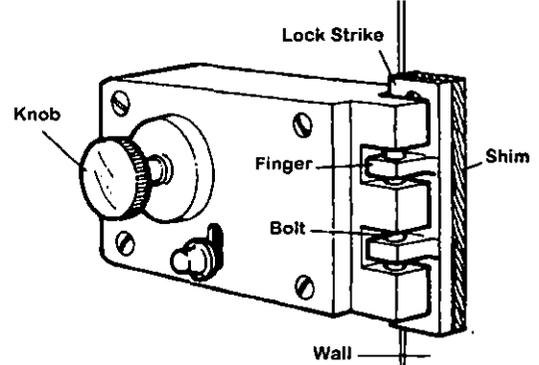
**4. Install the latch case,** securing it to the door with screws. The cylinder and tang should fit perfectly. Next, install the lock strike to the jamb of the door. You may have to shim it so the lock fingers meet the bolt. Try the lock to be sure it operates, then tighten all screws.
