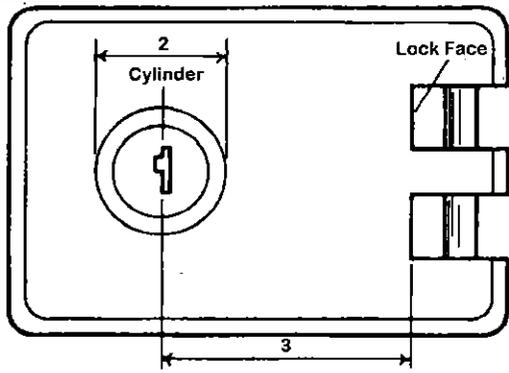
**1. Surface-mounted vertical deadbolt** is one of the best locks you can buy. To locate cylinder hole, hold lock to door and (1) add the dimension to half (2) the diameter of cylinder. Both measurements combined (3), is distance to place the lock in from the edge of the door.
