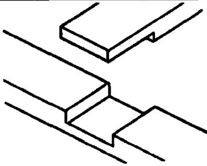
**Middle-laps** goes across the end of one piece of wood and through the face of the joining piece.
