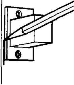
**3. Measure and mark** for the latch bolt, which has to be mortised into the door with a butt chisel. The depth of the mortise is the thickness of the latch plate. Go easy with the chisel, taking small cuts; latch can be shimmed if you make the cut a tad too deep.
