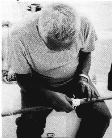
Here I am repairing the Commodore's boat brush handle with a 5B X 6L ordinary turkshead knot.
