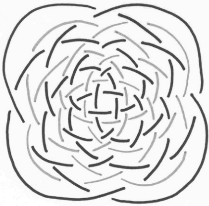
Fig. 7 - Spherical Covering Knot (first method), started with a 4B x 7L Turk's Head knot, similar to Ashley's knot #2219
