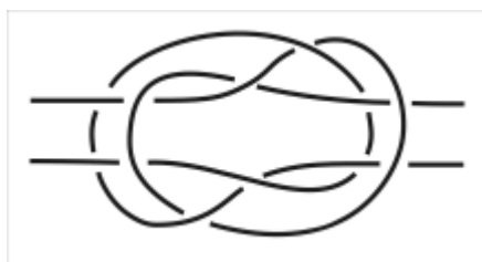
Figure 1 - Knot diagram of the jug sling
