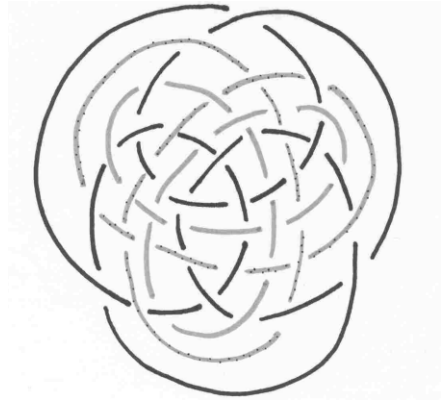
Figure 2. Completed drawing of a Spherical Covering Knot classified as a '3B x 4L, two cords added, inside.'
