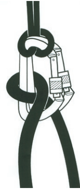
5b The Garda knot (Alpine clutch or Gardaknoten) The load is on the left-hand side.
