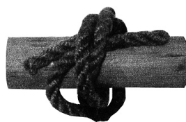
3. Round again and this time keep to the right hand side of the standing end and through and there you have it. (The mystery solved?)
