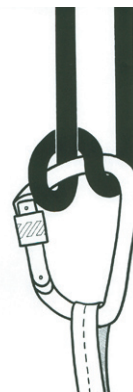
4b The Münster hitch (slant D-carabiner)
