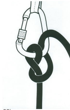
22b The Goulet Eight Münter hitch
