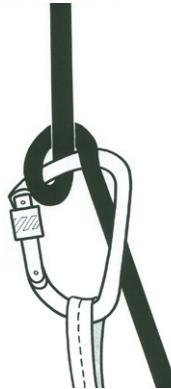
15b Münter hitch - braking side of rope over spine
