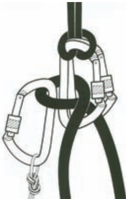
29 A Garda knot release technique A third carabiner with an accessory cord is clipped to the loop wrapping the spine. Pull down on the cord to release the Garda. Caution: the load is hard to control when released.
