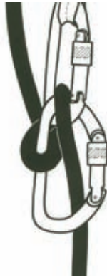
40d Improper braking method with the carabiner wrap belay The wrong side of the rope is being used to brake.
