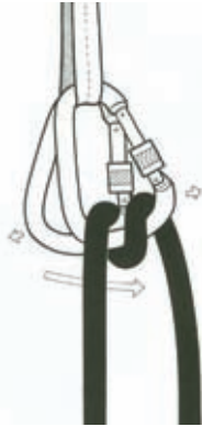
28b Garda failure - method 3 The HMS carabiners pivot apart and the rope slips. Once again, the carabiners are not secured with a girth hitch.
