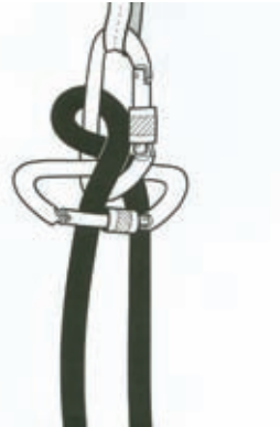
37c The C & F belay hitch with the gate opening downward Note that the load is on the left-hand side of the line.
