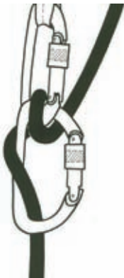
40a Proper braking method with the carabiner wrap belay
