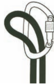
39a Setting up the carabiner wrap belay from scratch - step 1 Wrap a loop through the carabiner and around the spine.
