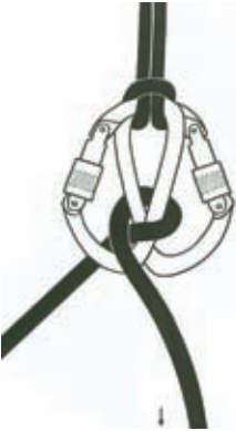
31a The Gelichlaufsperrre Follow the transition from 31a to 31b to 31c to 31d and back to 31a.
