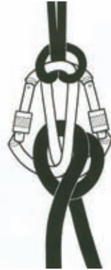
32 Gleichlaufsperrre failure The hitch can shift into something that resembles the Mnter hitch, and the rope will not lock up.
