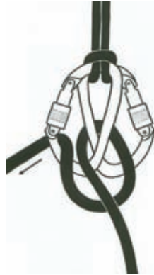
31d Re-clipping the Gleichlaufsperrre Follow the transition from 31a to 31b to 31c to 31d and back to 31a.
