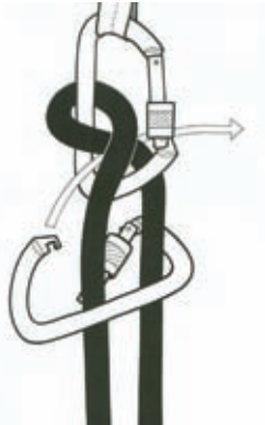
37b Setting up the C & F belay hitch - method 2 Clip the lower carabiner, as shown.
