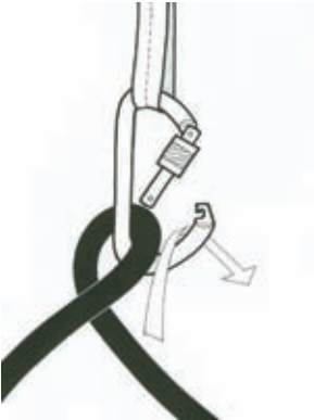
37a Setting up the C & F belay hitch - method 2 Wrap the slack side around the spine, and under the load side, and clip it in.
