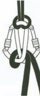
33 The Gegenlaufsperrre This hitch offers inconsistent performance and reliability.
