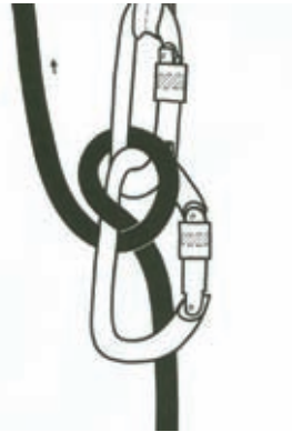
40e Improper braking method with the carabiner wrap belay The correct side of the rope being used, but it will get pinched by the load-bearing side.
