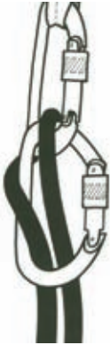
38c The carabiner wrap belay The left side of the rope is the load-bearing side, and it is in the non-braking mode.
