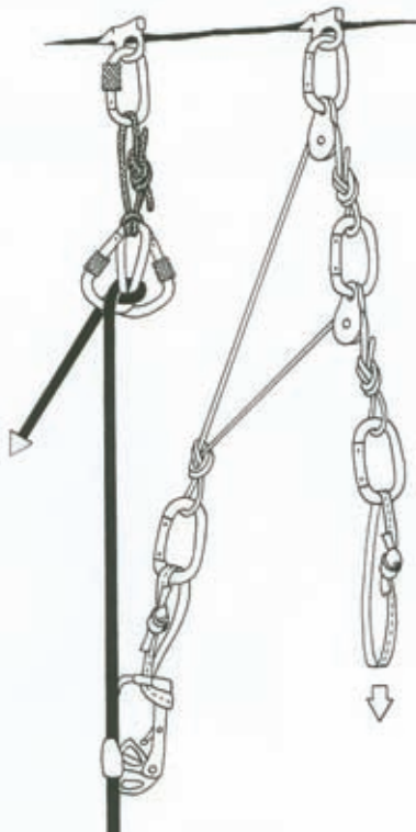
6a Garda knot with a detachable haul system The Garda knot can act as a locking belay or progress capture with improvised hauls. In this case, a detachable 3:1 inverted piggyback is depicted with a mechanical ascender and pulleys.
