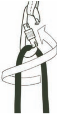
36a Setting up the C & F belay hitch - method 1 Wrap the load side of the rope behind the upper carabiner and clip it in.
