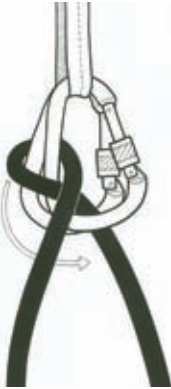
28a Garda failure - method 3 The bight wrapping the carabiner spines slips down.
