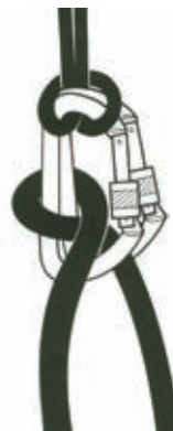
5b The Garda knot (Alpine clutch or Gardaknoten) The load is on the left-hand side.
