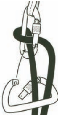
36b Setting up the C & F belay hitch - method 1 Clip the lower carabiner, as shown
