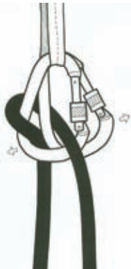
27 Garda failure - method 2 The rope can slip as the carabiners pivot apart. Note that there is no girth hitch securing the HMS carabiners.
