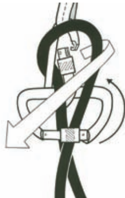
38b Converted the C & F belay hitch to the carabiner wrap belay Unclip the load-bearing side of the rope from the upper carabiner, and rotate the lower carabiner so the load-bearing side of the rope wraps the spine and not the gate.
