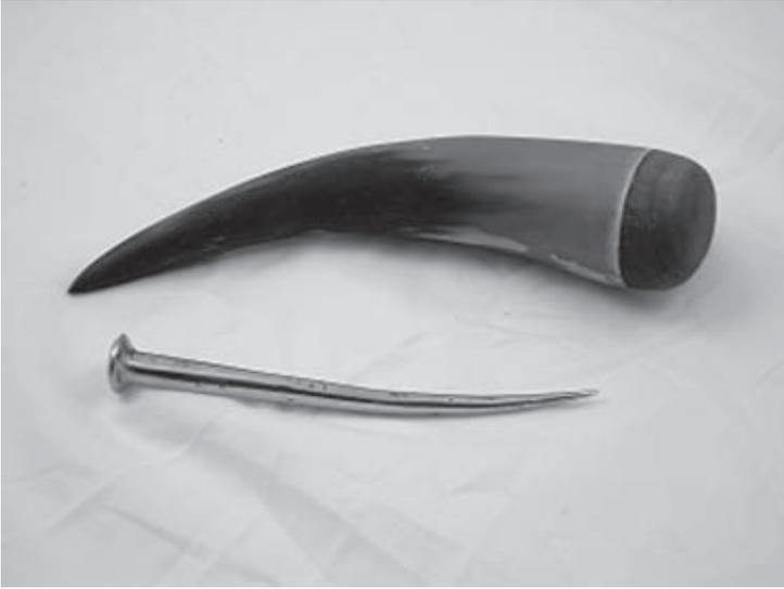
The illustration on the left shows reproductions of two significant early rope working tools, the "cow horn fid" and the possible evolutionary leap of the marling (marline) spike from the spikes shown in photo 2.
