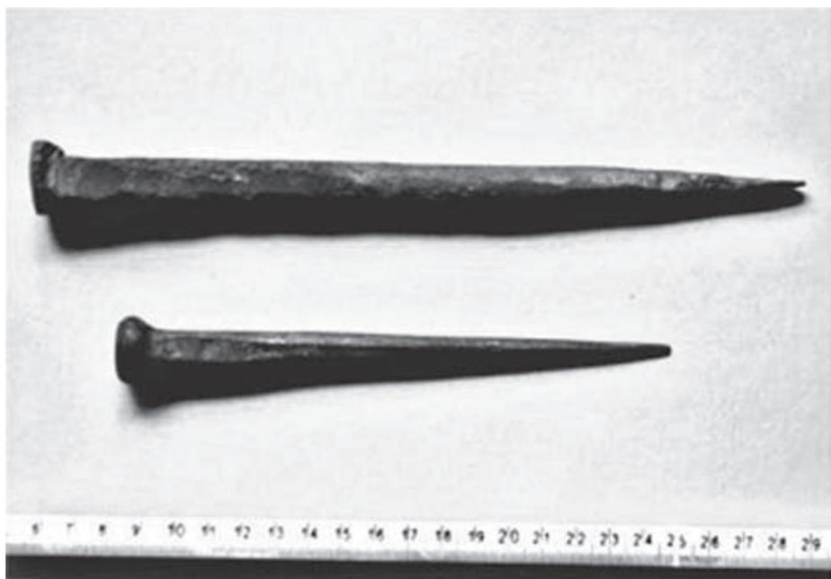
*These two boat spikes show the possible evolution of the boat spike to the marling spike. This was done by slightly beating down the edges in the fore end of the nail to something that is more comfortable to use and easier the handle. The lower example is a more refined version.*
