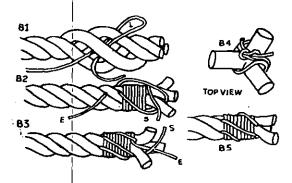
First open the strands near the end of the rope to be whipped, if possible, without unlaying the ends. Place the end of the twine between two strands of the rope, pass it around the third strand, and bring it out again between the strands through which it entered, B 1.
