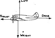
Opposing the weight is the "lift" pro-vided by the mainplanes passing through the air. In level flight "lift" and "weight" balance each other. The centre of lift is arranged to be bind the centre of multiple that it the
