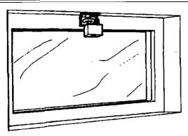
Basement windows (hopper type) that open from the top can be cecured with a hasp and padlock, as illustrated. Use one-way screws to attach the hasp; this way there is no chance a burglar can break the glass and remove the hasp, if the hasp screws are exposed.
