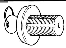
4. Screw in the cylinder from the exterior of the door. Special set screws will hold it in position so it can't be removed by a burglar. Then install the strike plate on the doorjamb for the latch bolt. Sometimes, this lock requires only a drilled hole in the jamb to accept the bolt.
