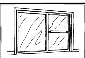
A burglar bar on patio windows is deterrent, but a burglar can still force the lock and jimmy the door. Use a burglar bar in combination with the screw trick shown above, plus a window lock. The burglar bar is hinged on one end; there is a width adjustment on the other end.
