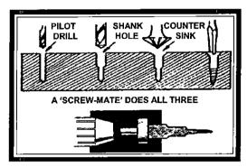
To drive screws easier, pre-drill pilot holes for them about the same diameter as the threads of the screw. If you are countersinking, pre-drill the pilot hole then countersink it. You can also slide the screw threads over soap or beeswax to make them easier to drive—especially in hardwoods. You can buy countersinks for portable electric drills and stationary drills that, at one time, drill the pilot hole, shank the hole, and countersink the hole.
