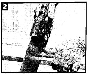
Use your thumb on the side of the blade to steady it when starting a cut. Make short pull strokes on the waste side of the line.
