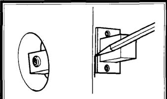
3. Measure and mark for the latch bolt, which has to be mortised into the door with a butt chisel. The depth of the mortise is the thickness of the latch plate. Go easy with the chisel, taking small cuts; latch can be shimmed if you make the cut a tad too deep.
