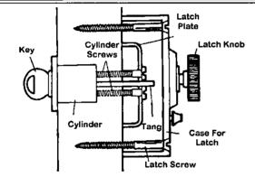
3. Anatomy of a surface-mounted deadbolt shows how the cylinder and tang fits through the door and into the backplate and lock. The cylinder is secured in the door by the tang and the backplate, plus two screws driven through the backplate into the back of the cylinder.
