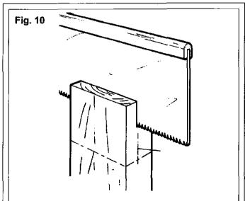
To cut a rabbet joint by hand, use a backsaw guided along penciled cut-off lines. The width of the cut is half the wood's thickness.
