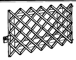
An accordion gate offers maximum protection for basement windows, yet is fairly easy to open from the inside in the event of an emergency. The gate is padlocked with a hasp. You also can buy burglar bars or grills that are set into the jambs of the windows.
