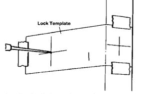
1. To install a deadbolt, use the manufacturer's template to locate the hole positions. Tape the template to the door about 10 ins. above the lockset.- use a square to make sure that it is square on the door. Before buying, measure door thickness; locks vary.
