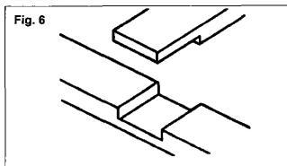
Middle-laps goes across the end of one piece of wood and through the face of the joining piece.
