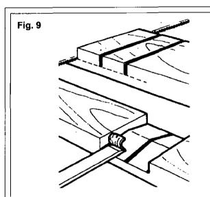
With a sharp chisel, remove the access wood between the saw cuts, as illustrated. Smooth the bottom of the cut with a rasp.
