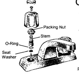
ost leaky compression faucets need new seat washers. Pry off the decorative cap on the handle, remove the handle screw, pull off the handle and use a crescent wrench to unscrew the packing nut. After unscrewing the stem, remove and replace the seat washer held in place by a brass screw. Coat the washers with nontoxic, heat-proof plumber's grease. Pop the stem out of the
