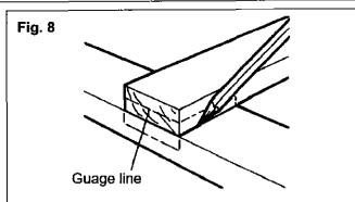
Mark wood to guide saw for lap joint and then make cut. Or use dado blade in power saw.
