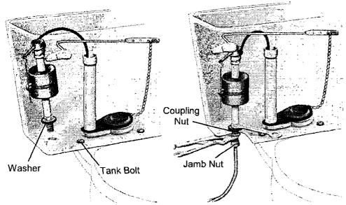
IF THE BALL-COCK WASHER has hardened or if the ball cock leaks, start by replacing the washer (above left). If the leak persists, replace the entire ball cock. Use an open-end wrench inside the tank and self-locking pliers outside (above right).
