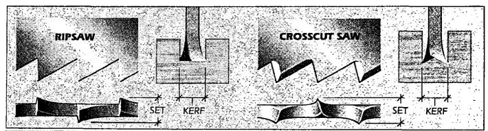
Ripsaws are designed for cutting parallel to the grain and have chisel-like teeth that plow through the wood. Crosscut teeth are pointed to sever wood fibers. Both types of teeth are bent out, or set, to create a kerf that's wider than the blade.
