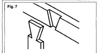
**Dovetail-lap** is a fancy joint where appearance is important. Cut it by hand or with a power saw.
