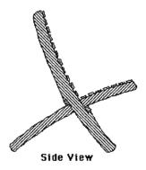
These plans are based upon several designs used by scouts. Some people call this a scissors chair. The chair is composed to two pieces: the seat and the back. The two pieces slip together and require no fasteners when used. When carried the seat stows between the sides of the back for a very compact package.
