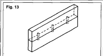
Edges of board must be perfectly square for perfect dowel joints. Apply glue to one end of dowels, then insert dowels into one board. Apply glue to the dowels and adjoining board and tap both pieces together. Clamp.
