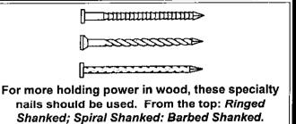
early days, the same abbreviation was used to indicate a pound in weight. Nails were weighed by the thousand, so if 1,000 nails totaled 12 pounds, they were 12d, or 12-penny nails. The penny system has endured, although today it refers only to nail length. For example, a 2d nail is 1 in. long; the length increases 1/4-in. for each higher number up to 10d. Then the penny system gets more complicated (see chart).
