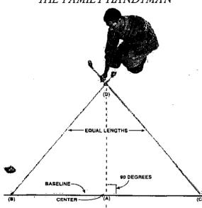
Unless you live in an igloo, you'll probably have to establish rightangle reference lines for one of your home improvement projects. Laying floor tile, building walls and laying patio bricks are a few examples of jobs requiring perpendicular layout lines to get started. The method we're showing is based on simple geometry, but you don't have to do any math to make it work.
