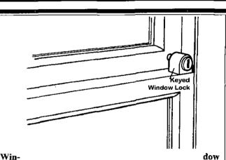
key lock is best lock type, since the burglar can't open the lock and would have to break the glass and the window mullions in order to get into the house. Some key locks are adjustable so you can crack the window for ventilation without activating the lock.
