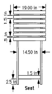
All pieces are cut from a strong hardwood like oak. The Seat Legs and Back Legs are cut from these pieces to formed curved pieces. The Seat Leg is 2" wide. The Back Legs are 2.5" wide except for regions that taper to 3" wide to form 1/2" backstops for seat supports. See the seat support detail.
