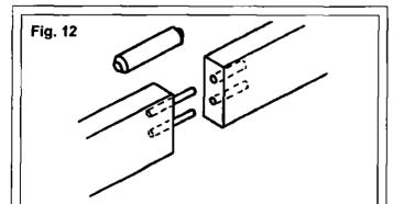
Dowels strengthen butt joints. You must use a stationary drill press or inexpensive doweling jig for this job. You can buy precut dowels with beveled edges and fluted sides which allow trapped glue to escape. End-to-end doweling is called a "splice". About half of the dowel is inserted in each end of the board, but leave room at the bottom of the holes you drilled for excess glue "well".
