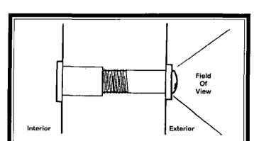
A peeper is a common security measure. It is a look-through glass with a wide angle range. You simply look through it to see who's knocking at the door. Installation in a solid core door is little more than a hole drilled in the center of the door at eyeball height. The outside section of the peeper is inserted through the hole from the outside and screwed into the inside section.
