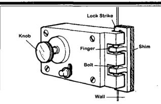
4. Install the latch case, securing it to the door with screws. The cylinder and tang should fit perfectly. Next, install the lock strike to the jamb of the door. You may have to shim it so the lock fingers meet the bolt. Try the lock to be sure it operates, then tighten all screws.
