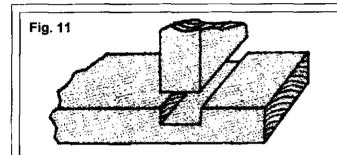
**Dado Joint** is used for joining shelves, boxes and drawers. It's stronger than a butt joint. The dado joint has limited application in rough construction.
