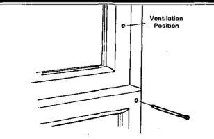
For double-hung windows, you can improvise a nail or bolt lock by simply drilling holes through the bottom frame of the window and into the top frame. The nail or bolt is inserted flush into the hole(s). You can space the holes so you can crack the window for air.
