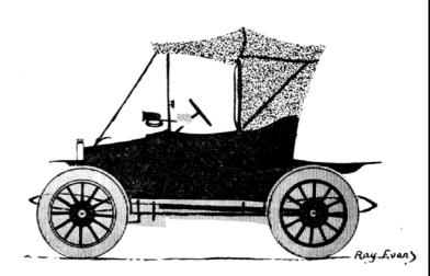
AUSTIN 1910 Austin 1910, forerunner of the famous "7" which was not actually produced until 1922. A single cylinder shaft drive, magneto ignition 7 horsepower engine with a Bore/stroke 105 × 127 mm. Internal brakes rod and cable to rear wheels.
