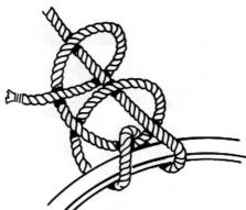
This is an excellent knot for attaching a rope to a light anchor, a ring or a rectangular piece of stone. It can also be used to rig up a swing.
