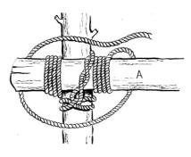
This lashing is used whenever spars cross at an angle, touching each other where they cross. The lashing starts with a clove hitch (or timber hitch) around the
