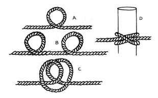
This is a most useful knot and is the start and finish of some lashings and is widely used in boat work, gadget making and pioneering and for making rope ladders. Passing around an object in one continuous direction, it puts almost no strain on the fibres.
