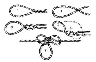
Pick up a bight of the rope in one hand and hold both parts in the other Fig. 1. Twist the bight once to cross the two parts Fig. 2, twist again to produce hole A Fig. 3. Fold bight back over loop passing tip down between the two parts C and up through A Fig. 4, now pull bight through and tighten knot.
