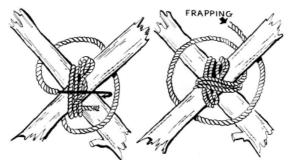
This lashing is used to "spring" two spars together. The lashing is started with a timber hitch around both spars. The timber hitch is tightened so as to draw the two spars together. Three or four turns are then taken around one fork, and three or four turns around the other fork. Two frapping turns are taken about the lashing at the point where the spars cross, and the lashing is finished off with a clove hitch around the most convenient spar.
