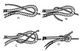
The sheet bend is the most important knot for joining two rope ends and is especially useful when the ropes are of unequal size. A permanent loop - tied, seized or spliced - can be substituted for the right hand portion of the knot.
