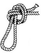
To make a loop in the end of the rope use this knot. It can be tied quickly but if a great deal of tension is placed on it it tends to jam.
