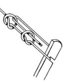
As its name suggests this knot is used in securing tent guy lines or guys for pioneering projects and larger gadgets. It is started by casting two overhand knots in the rope some distance apart, the running end is then passed around the peg, carried upward, then down through the two overhand knots. The knots
