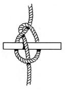
This knot can be used as a quick method of getting a purchase in a rope for pulling. It is so named because a marlin spike, or small spar is run through a loop as illustrated.
