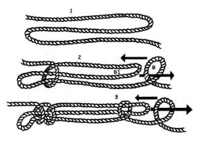
This knot is used for shortening a long rope which is fastened on both ends. As in the case of a tent guy line or blanket line. After taking up the slack as shown in Fig. 1 form an underhand loop as shown in B, slide it over the bight B 1, and pull it taut. Do the same thing on the other end to complete the knot. To lock the sheep shank to keep the loops from sliding off add a second half hitch as in Fig. 3 at each end.
