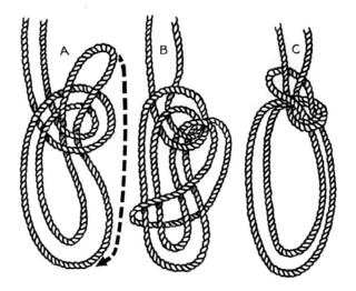
This knot is used as a chair knot. Form a good size bight and throw an overhand loop as shown in Fig. A, bringing the ends up through the loop so formed. Open the end loop and bring it down and around the entire knot as shown in Fig. B, until it ends up against the standing part as shown in Fig. C. Set the knot securely before putting weight on it.
