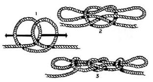
Adjust the two loops at this stage in order to pass around a body. One, the smaller will allow it to pass over the head and shoulders and rest under the arms, with the knot near the chest - the other long enough to go under the knees.
