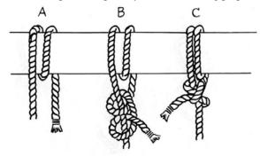
The round turn is shown in Fig. A and means that the rope makes two turns around the spar. You can see in Fig. B that the second half, the two half hitches is like making a clove hitch on the standing part of the rope with the free end. Pull tight at this stage and it will then look something like B. Sometimes the free end is fastened with a light whipping to the standing part for greater security.
