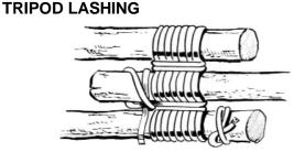
To lash three spars together to form a tripod, lay the spars on the ground pointing in alternate directions. Begin with a clove hitch or timber hitch on one of the end spars. Take seven or eight loose lashing turns around all three spars and loose frapping turns in the spaces between. Finish with a clove hitch on the centre spar and hoist the tripod.
