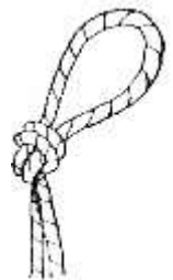
An Overhand knot, also for making a big loop, is a lubber's knot, which is very easy to tie, but difficult to undo again.
